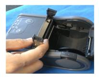
When using the label peeler issuing mode: Peel off the first label, and press the peeler change over lever to lift the peeler holder.
